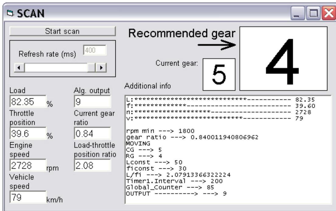
Fig. 6 Software output window of the model executive phase (algorithm) with recommended gear
