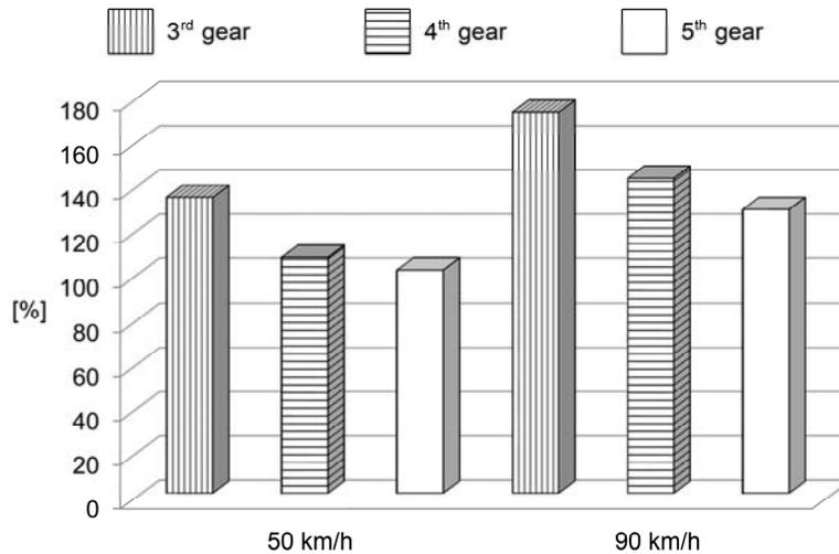
Fig. 1 Fuel consumption related to 50 km/h in 5th gear
