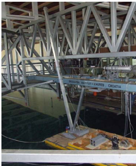
Fig. 3 - Physical model in the towing tank
