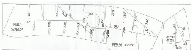
Figure 2. Plate with nesting plan providing test specimens
