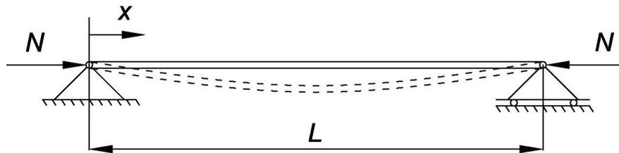
Fig. 3 Beam buckling
