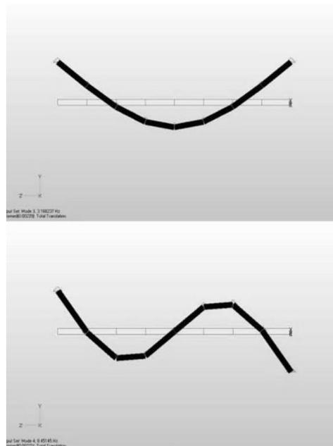
**Fig. 2** The first and the second natural mode of beam vertical vibrations, NASTRAN
