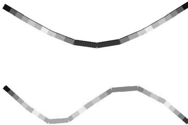
**Fig. 1** The first and the second natural mode of beam vertical vibrations, SESAM
