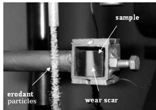
*Figure 4 Testing of solid particle erosion*
