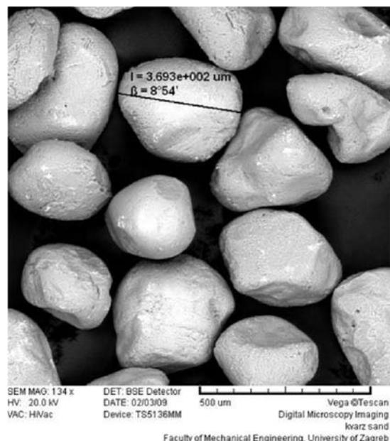
*Figure 5 Erosion particles of quartz sand*
