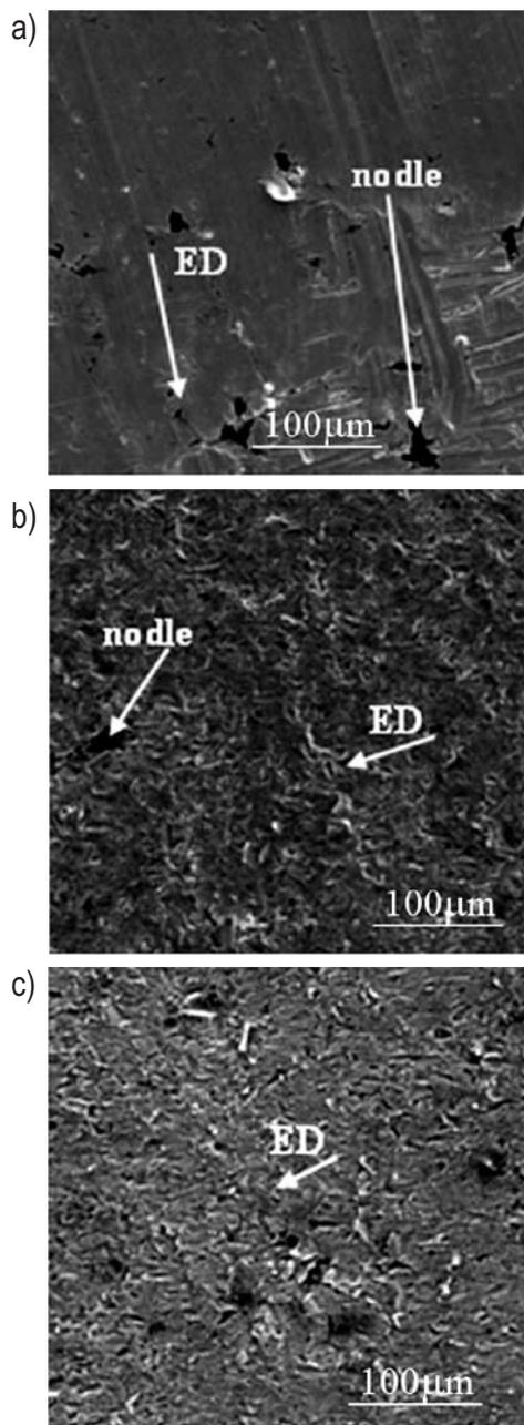
**Figure 9** Sample surfaces of ductile iron eroded at impact angle:
