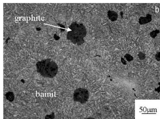
Figure 2 Samples of a) ductile cast iron, b) austempered ductile iron
