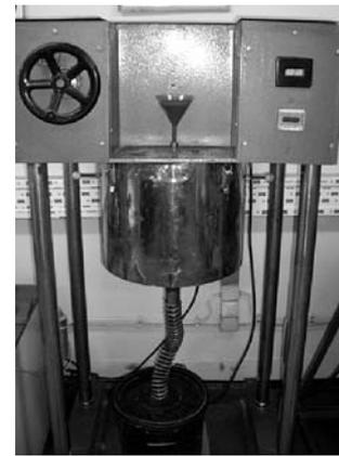
*Figure 3 Particle erosion tester*
