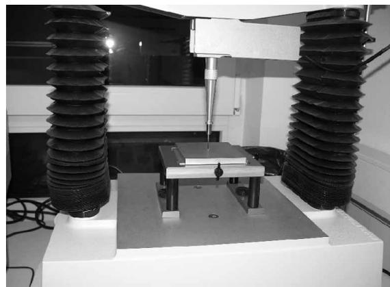
Fig. 3. Indentation testing of the rat femur.
