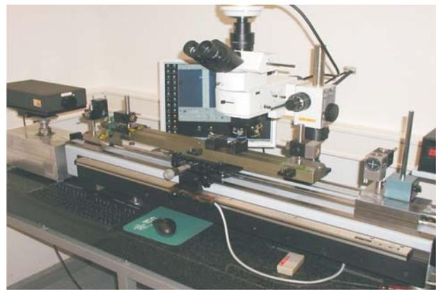
Figure 1 System for calibration of precise line scales
