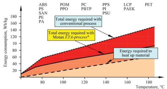
FIGURE 13 – *ETA*-process energy consumption<sup>18</sup>
