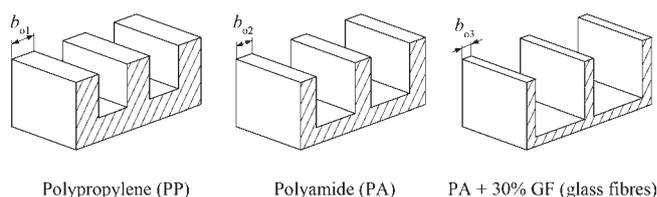
FIGURE 4 – Comparison of moulded parts wall thickness with different materials<sup>6</sup>
