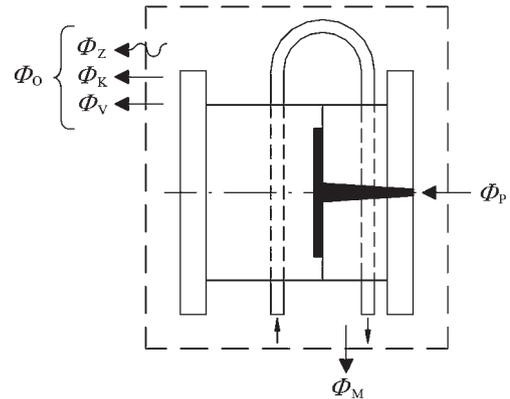
FIGURE 6 – Mould – heat exchanger:  $\Phi_p$  – heat that thermoplastic melt brings to the mould,  $\Phi_o$  – heat exchanged between mould and the environment,  $\Phi_z$  – heat exchanged by radiation,  $\Phi_k$  – heat exchanged by convection,  $\Phi_v$  – heat exchanged by conduction,  $\Phi_M$  – heat exchanged between mould and coolant<sup>7</sup>
