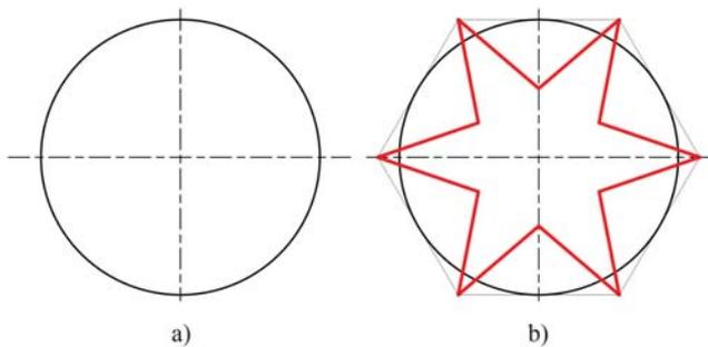
FIGURE 8 – Cross-sections of cooling channels: a - classic shape, b - shapes achievable by AM<sup>11</sup>
