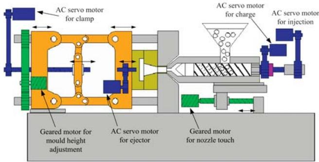
FIGURE 11 – Cross-section of all electric injection moulding machine<sup>16</sup>
