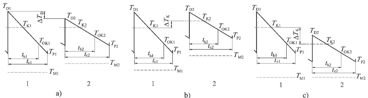
FIGURE 5 – Influence of mould material on moulded part cooling time: a - required cavity wall temperature, b - required contact temperature, c - required coolant temperature; 1 - material with lower thermal properties, 2 - material with higher thermal properties;  $T_D$  - contact temperature (K),  $T_{OK}$  - mould opening temperature (K),  $T_M$  - coolant temperature (K),  $T_P$  - start temperature (K),  $t_c$  - injection moulding cycle time (s)<sup>7</sup>
