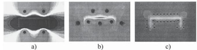
FIGURE 10 – Comparison of mould temperature fields: a - classic channels, b - optimized classic channels, c - *Contura*-system channels<sup>14</sup>
