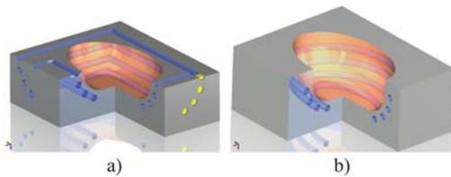
FIGURE 7 – Example of mould plate cooling: a - classic, b – conformal<sup>8</sup>
