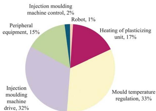
FIGURE 1 – Share of energy consumption in representative injection moulding system<sup>1</sup>
