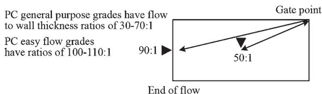
FIGURE 2 – Flow length – wall ratio for two grades of PC with equal wall thickness (1mm)<sup>4</sup>
