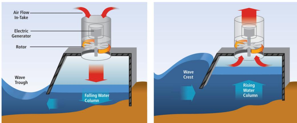
**Fig. 4.** Oscilating water column, [4]
