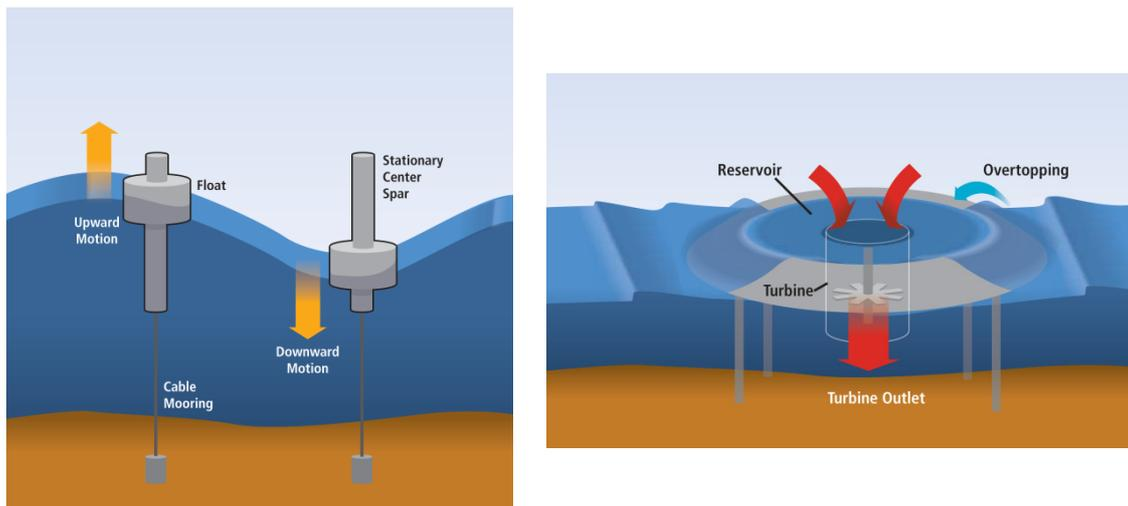
**Fig. 5.** Oscilating body and overtopping device, [4]
