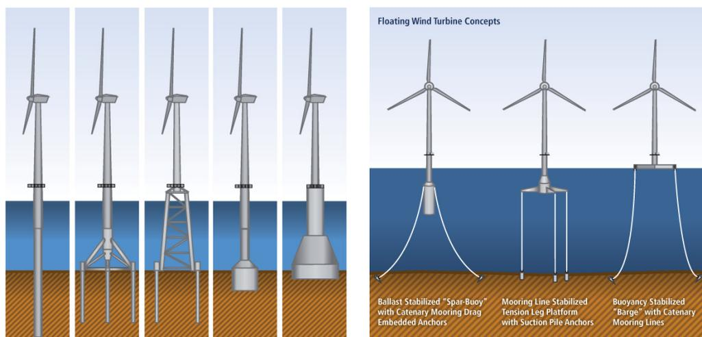
**Fig. 1.** Different types of fixed and floating offshore wind turbine supporting structure, [3]
