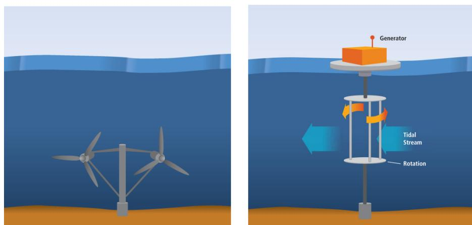
Fig. 2. An example of the horizontal and vertical axis tidal turbines, [4]
