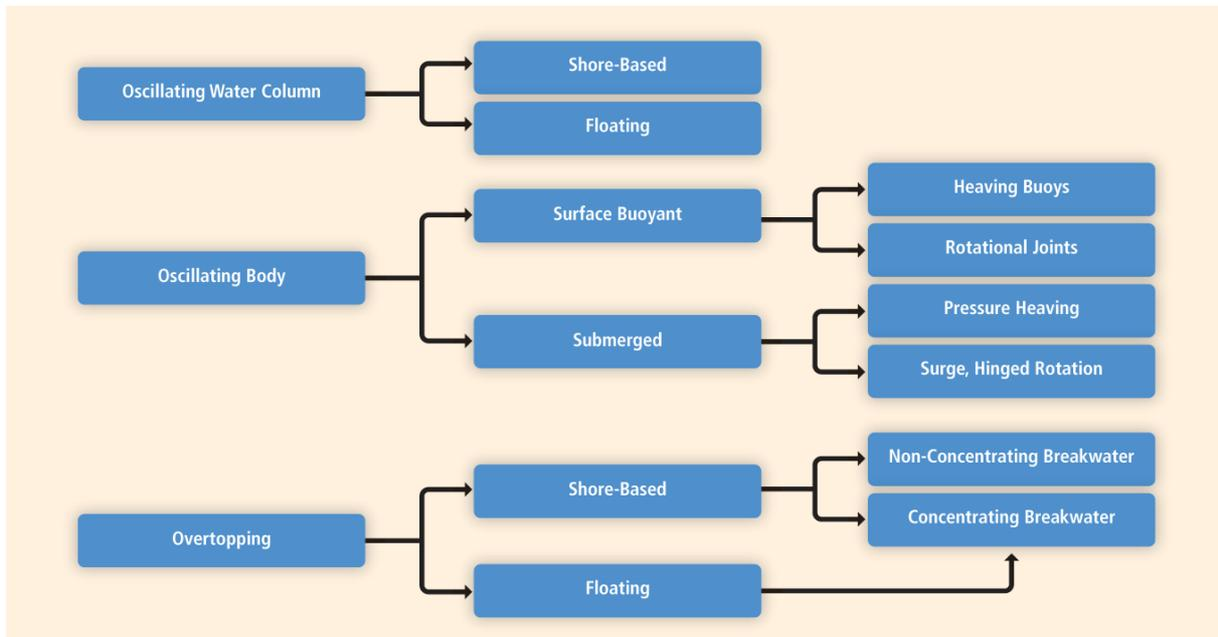
**Fig. 3.** Classification of wave energy converters, [4]
