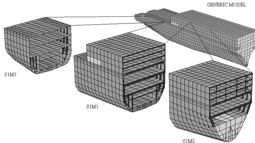
Fig. 6 MAESTRO 3D generic model of RoPax ship
