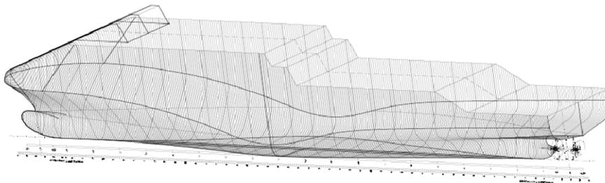
**Fig.3** Body Lines of RoPax (Level II)
