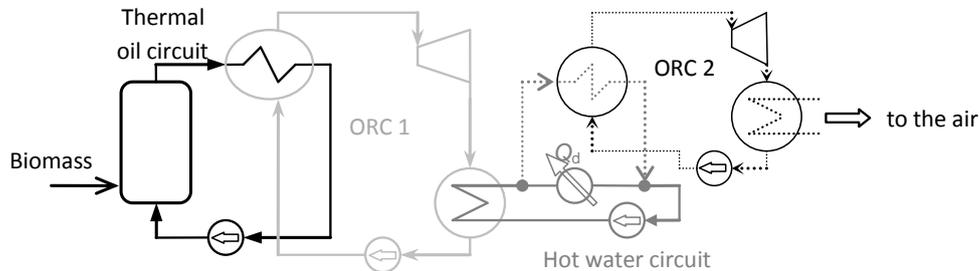
Figure 3: Simplified configuration of two ORC plant cascade
