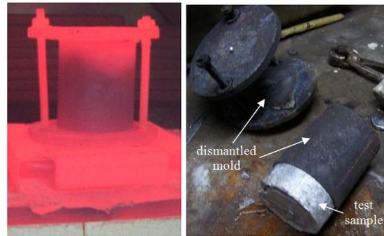
**Figure 3** - The process of producing aluminium foam samples
