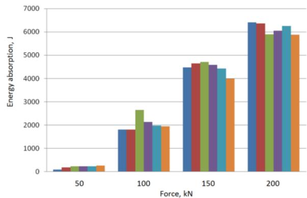
Figure 9 – Energy absorption of aluminium foams with equal dimension and density ( $\rho = 0,81 \text{ g/cm}^3$ )
