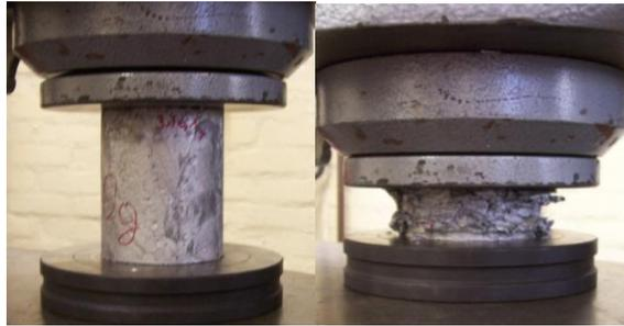
Figure 5 – Compression of aluminium foam sample
