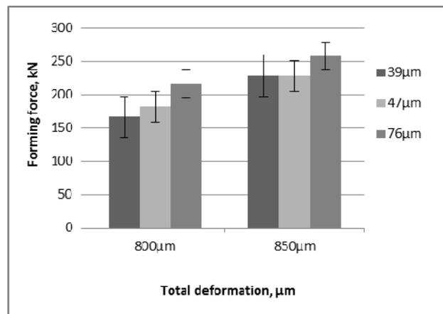
*Fig. 3 - Relation between forming force and total displacement - closed die coining*
