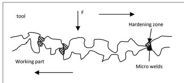
**Fig. 7 - Bowden and Tabor adhesion model [3]**
