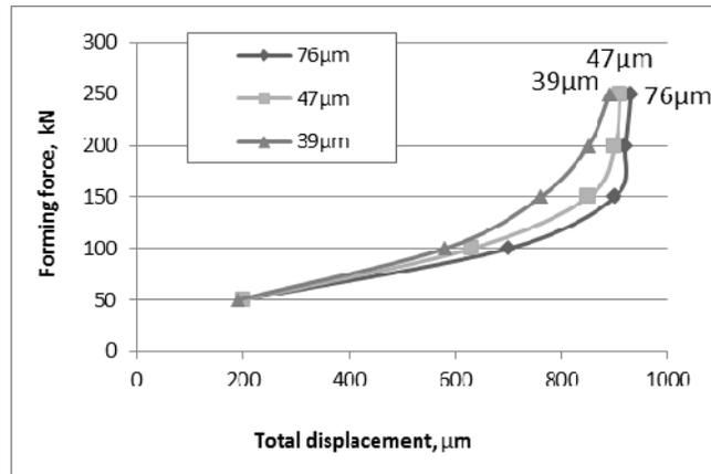
*Fig. 2 - Relation between forming force and total displacement - open die coining*
