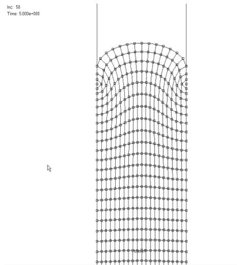
**Fig. 5 - Distorted mesh at the end of coining process**
