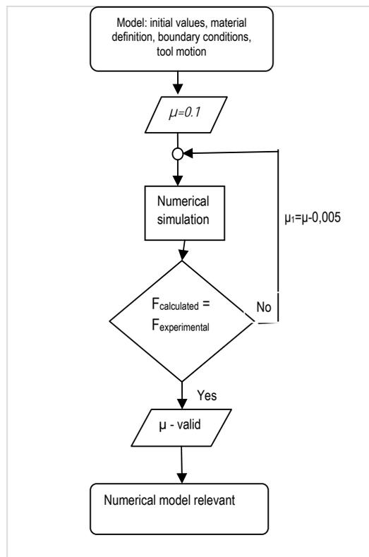
*Fig. 6 - Algorithm used for numerical determination of friction coefficient*
