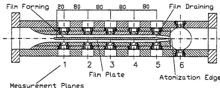
**Figure 1.** Schematic representation of the test section [27]
