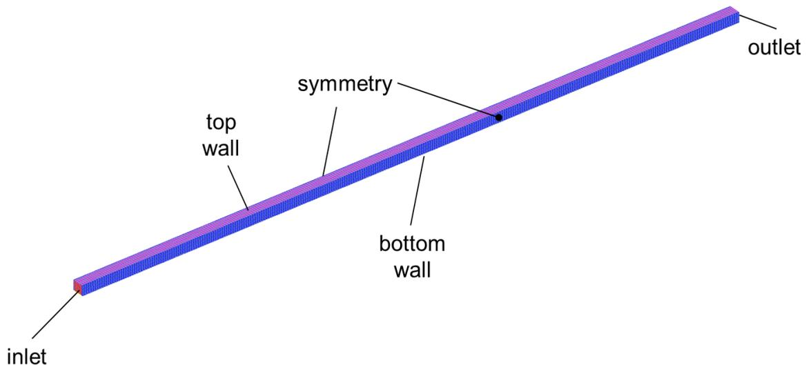
**Figure 2.** Mesh representation of the computational domain
