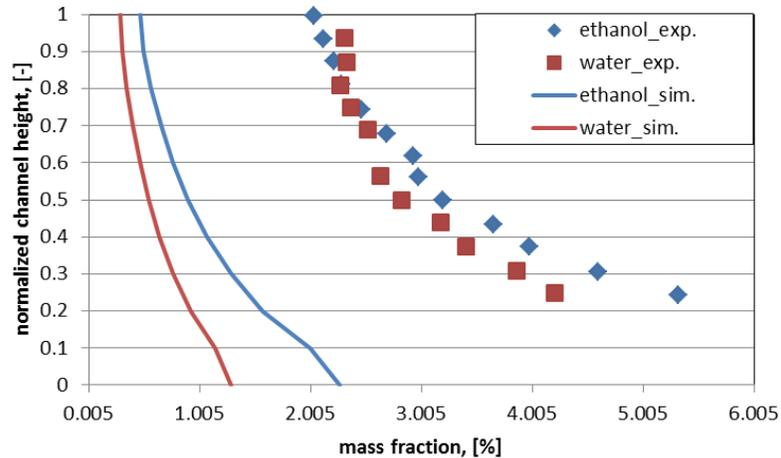
**Figure 4.** Comparison of gas phase concentrations in measurement plane 4 (O'Rourke model)
