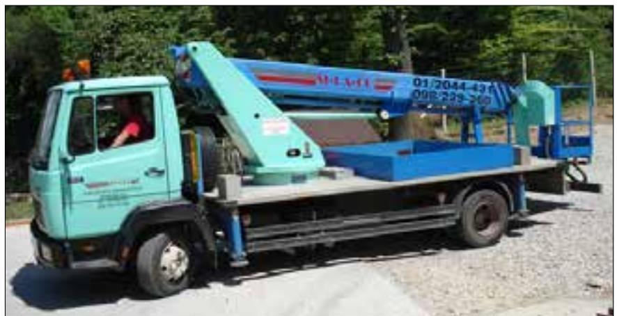
**Figure 1.** Mobile hydraulic platform Wumag WT 225
