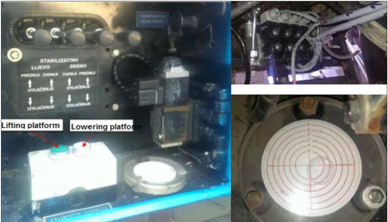
**Figure 3.** Cabinet for automatic levelling after reconstruction procedure, hydraulic distributors for nivelation process and circular libelle
